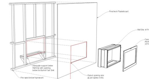
**IMPORTANT** Insulation must be securely wrapped around the firebox body before placing inside opening
