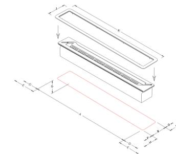
Slimline's unique Mounting Frame enables a clean, flush finish into the bench surface.
